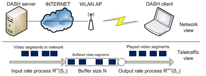
Fig. 1. System model: network and teletraffic view.
