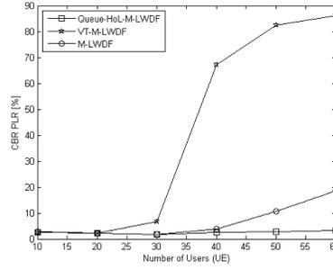
(b) Packet loss ratio for CBR flows
