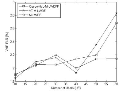
(c) Packet loss ratio for VoIP flows
