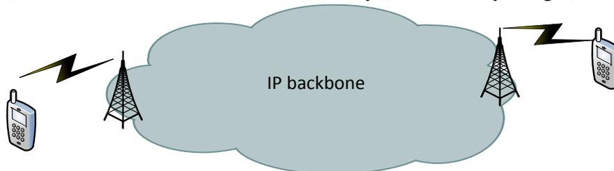
Figure 2 - Network scenario used for the LTE single hop maximum delay evaluation.
